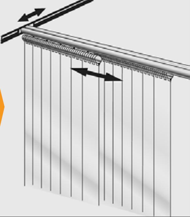
The diagram shows two curtain panels hanging from a track. The track is mounted to a horizontal ceiling. The curtain consists of a series of vertical slats or pleats. Arrows indicate that the two panels can be moved horizontally along the track.
