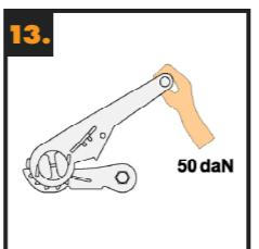
**OVERLOADING** - Web lashings shall not be overloaded: Only the maximum hand force of 500 N (50 daN on the label; 1 daN = 1 kgf) shall be applied. Mechanical aids such as levers, bars etc. as extensives are not to be used unless they are part of the tensioning device.
