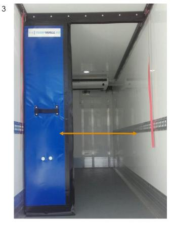
The panels can move from left to right to create an opening of 1/3 or 2/3 of the width.
