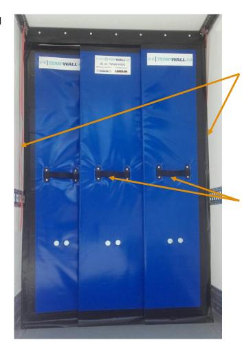
The Cool67 TopMounted 3D is in closed position with the floor locks on.
