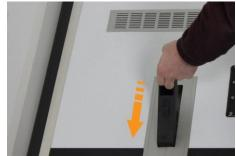
Date : Oct-2024 Version : 1.1 Release the floor locks by pulling the black handles into the down position.
