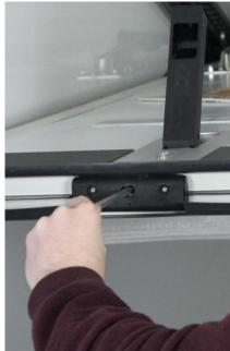
If necessary, adjust the ground stops using an allen key (10 mm) at the bottom.
