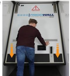
Once the bulkhead is in the desired position, close it downward into the vertical position.
