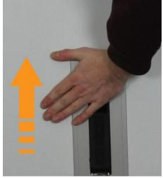
Once the Frigo58 is in the down/vertical position, close the floor lock handles as shown. The floor locks are only engaged when the black handles are flush with the bulkhead. Your Frigo58 is now secure.
