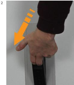
Date : Oct-2024 Version : 1.1 Release the floor locks by pulling the black handles into the down position.
