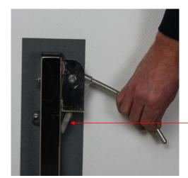
Adjust the height of the rubber floor stop.
