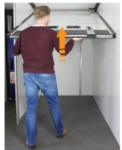
Lift the Frigo58 in a horizontal position against the roof.
