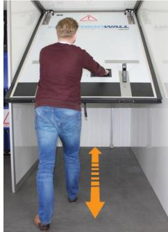
You can now move the bulkhead backwards or forwards into the desired position by simply pushing or pulling whilst it remains at 45 degrees.
