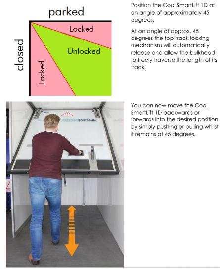
Position the Cool SmartLift 1D at an angle of approximately 45
