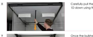
Carefully pull the Cool SmartLift 1D down using the belt.
